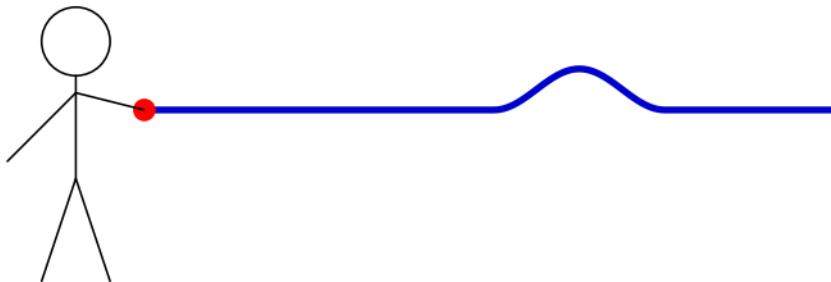
The speed of the wave depends on the tension on and mass of the string.
