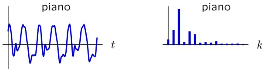
For example, the time function highlights periodicity, while the Fourier series highlights the distribution of energy across frequency.
