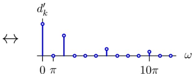
Compressing the time axis has stretched the  $\omega$  axis.
