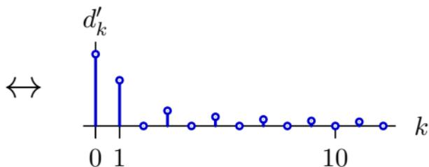
Compressing the time axis has no effect on the coefficients' dependence on  $k$ . Only the fundamental frequency has changed.
