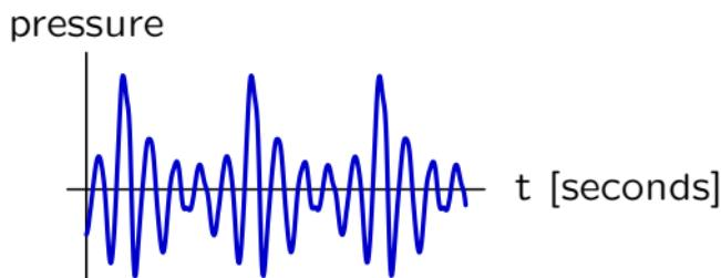
Although this time function is a complete description of the sound, it does not expose many of the important properties of the sound.
