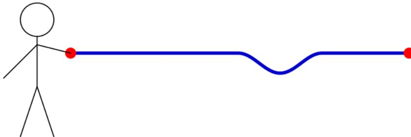
The amplitude of the reflected wave is opposite that of the incident wave.
