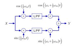
Assume each LPF is ideal, with cutoff frequency  $\omega_m/2$ , and DC gain of 2. Also assume that the input signal has the following Fourier transform.
