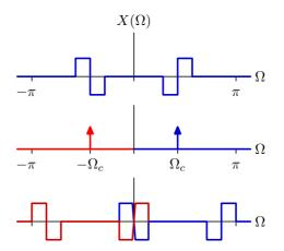
When we multiply by  $\cos(\Omega_c n)$ , the red and blue parts cancel near  $\Omega = 0$ . After the second multiplication by  $\cos(\Omega_c n)$ , the result near  $\Omega_c$  is zero!
