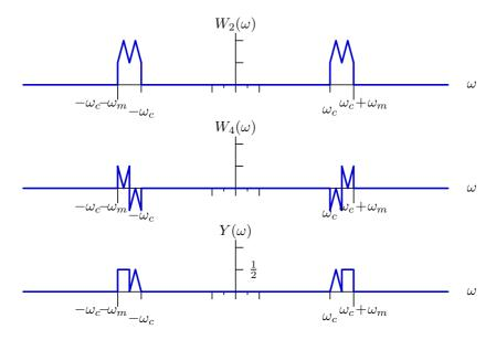
Notice that the frequency components of  $Y(\omega)$  are near  $\omega_c$  (not 0). Thus this scheme could be used to modulate a low frequency signal so that it can be transmitted via a high-frequency medium.
