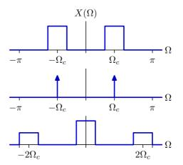
Multiplying x[n] by  $\cos(\Omega_c n)$  reproduces the components near  $\Omega_c$  at  $\Omega = 0$ . If we then LPF and multiply again by  $\cos(\Omega_c n)$ , we get back the original  $X(\Omega)$ . The system works like a bandpass filter.
