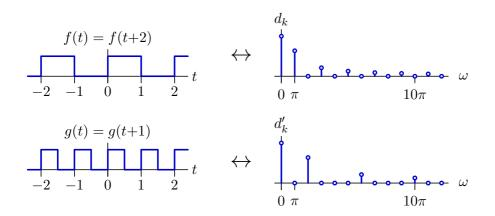
Compressing the time axis has stretched the  $\omega$  axis.
