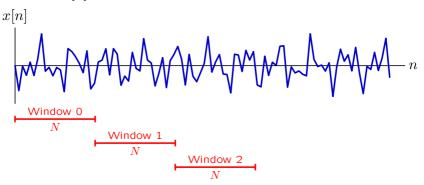
Filter data **in each window** by computing its DFT and zeroing components outside passband.
