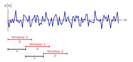
If the length of  $h[n] \leq N-s+1$ , then the length of h[n] convolved with s samples of the input will be less than  $N \rightarrow \text{no circular convolution artifact.}$
