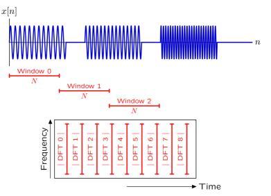
How would doubling the length of the analysis window  ${\cal N}$  affect the resulting spectrogram?
