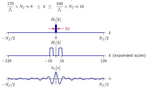
Zero-pad to make filter length equal to window length N = 8192.
