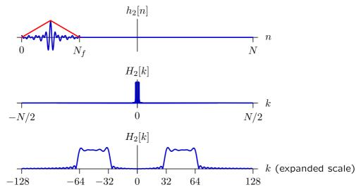
We can reduce the passband ripple by applying a triangular window.
