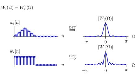
We can reduce the passband ripple by applying a triangular window (red).
