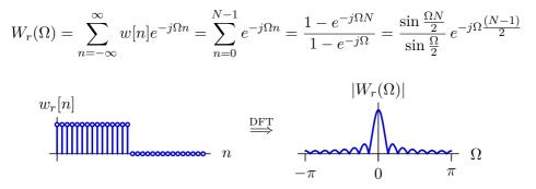
Multiplying the unit sample response h[n] by a window function, convolves the desired bandpass shape with the DT sinc – generating ripples.
