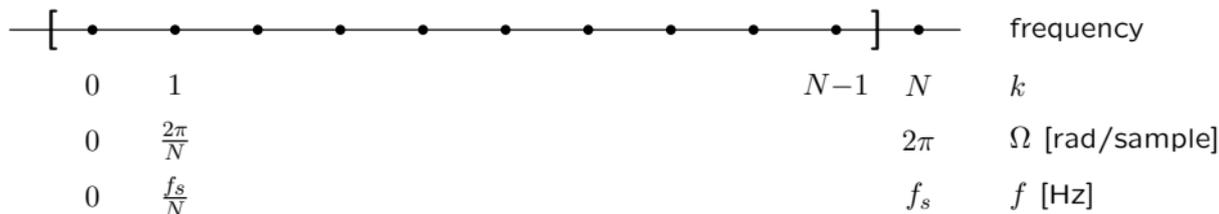
$N$  determines both the length of the window in time and the frequency resolution of the result.
