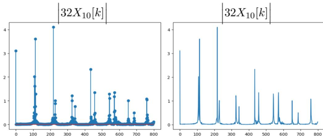
Clear peaks at  $k = 217$  and  $k = 228$  ( $f = 292.04$  Hz and  $f = 306.85$  Hz).
