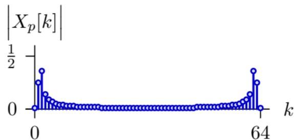
From this perspective, the large number of non-zero frequency components in the DFT of  $x_2$  are needed to generate the step discontinuity at  $n = 64$ .
