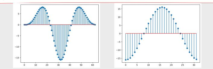
In this problem, one cycle of a sine wave with length 32 was convolved with itself. The result was greatest when the positive half cycles of the signals overlapped (n = 16) and smallest when the positive and negative halves overlapped (n = 32).
