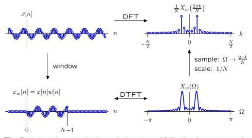
The finite length constraint is equivalent to multiplication by a rectangular window. What would happen if we used a different type of window?
