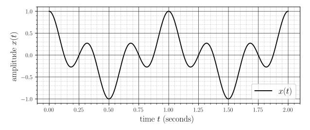
Suppose we sample x(t) every  $\Delta_2 = 0.5$  seconds — or, equivalently, with a sampling rate of  $f_2 = 2$  cycles per second (i.e., hertz) — to produce a discrete-time (DT) signal  $x_2[n]$ .
