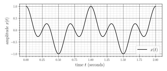
Suppose we sample x(t) every  $\Delta_1 = 0.25$  seconds — or, equivalently, with a sampling rate of  $f_1 = 4$  cycles per second (i.e., hertz) — to produce a discrete-time (DT) signal  $x_1[n]$ .
