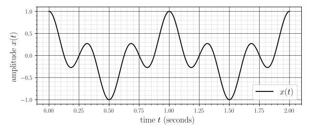
Suppose we sample x(t) every  $\Delta_3 = 1$  second — or, equivalently, with a sampling rate of  $f_3 = 1$  cycle per second (i.e., hertz) — to produce a discrete-time (DT) signal  $x_3[n]$ .
