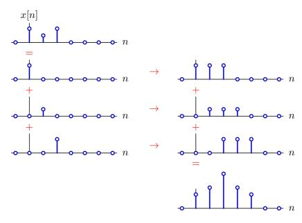
Superposition is easy if system is also  $homogeneous\ \mbox{and}\ time\mbox{-invariant}.$
