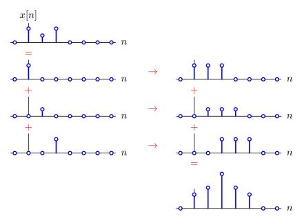
Response of a **linear** system is determined by its response to  $\delta[n]$ .
