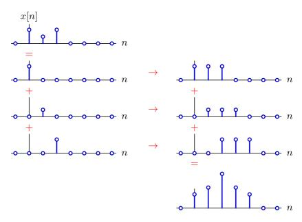
Superposition only works if the system is  ${\bf additive}.$
