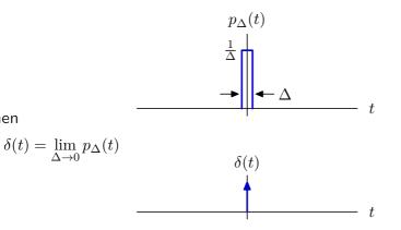
An arbitrary CT signal can be represented by an infinite sum of infinitesimal impulses (which define an integral).
