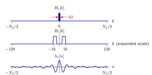
Zero-pad to make filter length equal to window length N=8192.
