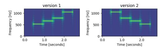
Version 1 clearly represents a sequence of tones with increasing frequency, while version 2 represents a sequence with decreasing frequency.
