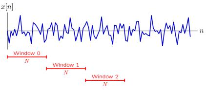
Filter data in each window by computing its DFT and zeroing components outside passband.
