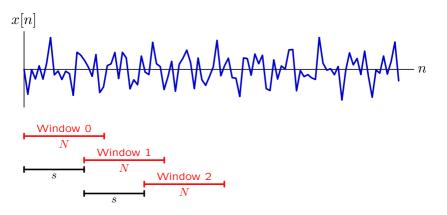
If the length of  $h[n] \leq N-s+1$ , then the length of h[n] convolved with s samples of the input will be less than  $N \to \text{no}$  circular convolution artifact.
