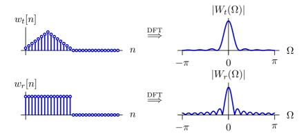
We can reduce the passband ripple by applying a triangular window (red).
