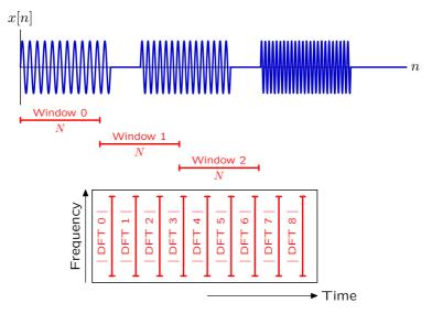
How would doubling the length of the analysis window  ${\cal N}$  affect the resulting spectrogram?
