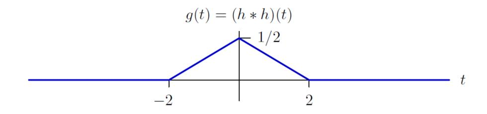
Convolution in time is equivalent to multiplication in frequency.
