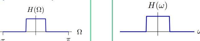
The **frequency response** is Fourier transform of **unit-sample/impulse response**!
