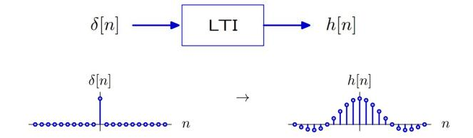
The unit-sample signal is the shortest possible non-trivial DT signal.
