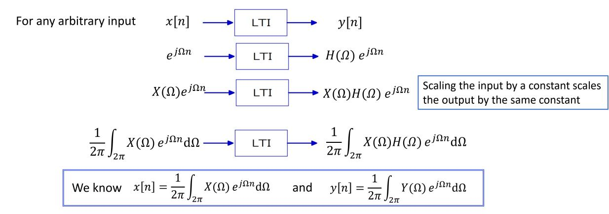
The Fourier Transform of the output,  $Y(\Omega)$ , can always be found by multiplying  $X(\Omega)$  by  $H(\Omega)$ .
