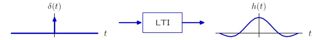
The response y(t) to a sinusoid  $x(t) = \cos(\omega t)$  is y(t) = (x \* h)(t).
