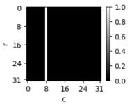
Array indices in numpy are [r,c], where r is row and c is column. The image is  $32 \times 32$  pixels. The bar is at c=8.
