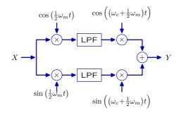
Assume that each lowpass filter (LPF) is ideal, with cutoff frequency  $\omega_m/2$ . Also assume that the input signal has the following Fourier transform.
