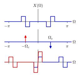
The cosine path preserves the part of the input  $X(\Omega)$  that is symmetric about  $\Omega = \Omega_c$ . The sine path preserves the part of the input  $X(\Omega)$  that is antisymmetric about  $\Omega = \Omega_c$ . Both are needed.
