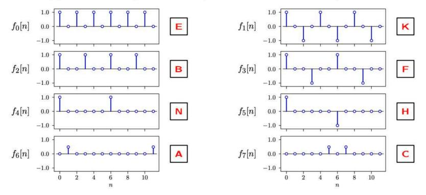
Determine which of the following plots (A-N) shows the real part of the 12-point DFT of each of the preceding signals ( $f_0[n]-f_7[n]$ ), and enter that letter in the corresponding box above. DFT values have been scaled/normalized (only match patterns)
