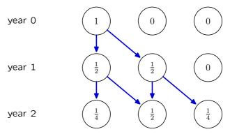
Since barrel #3 depends only on barrel #2, and barrel #2 depends only on barrel #1, the three barrel system is equivalent to the cascade of three one barrel systems!
