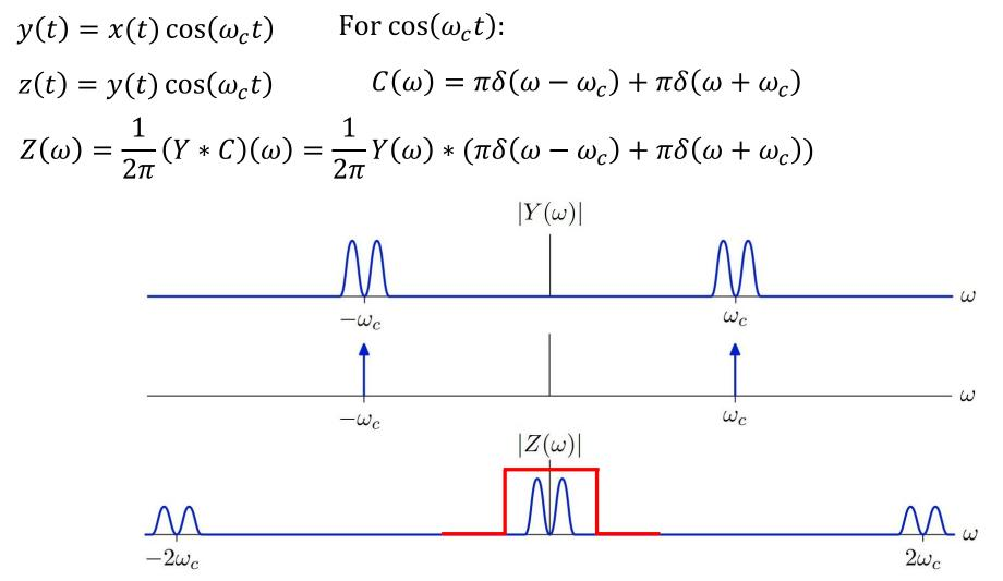
We can recover the original message by low-pass filtering:
