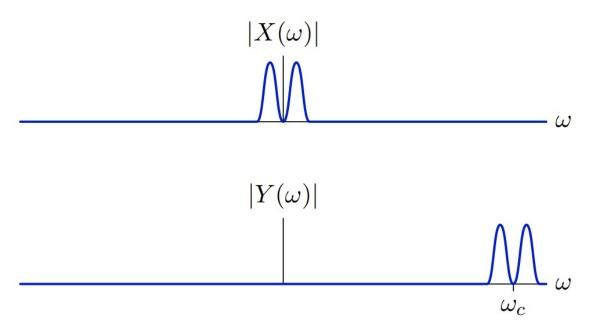
The problem with this idea is that the signal  $e^{j\omega_c t}x(t)$  has both real and imaginary parts – it is hard to be implemented physically.
