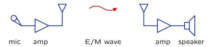
For energy-efficient transmission and reception, the dimensions of the antenna should be on the order of the wavelength.
