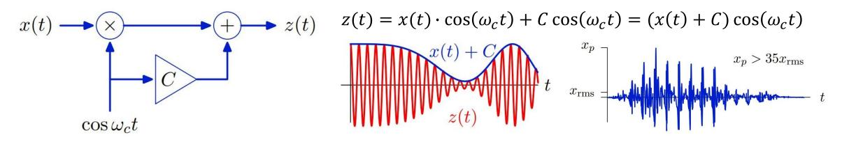
Adding carrier is equivalent to shifting the DC value of the signal x(t).
