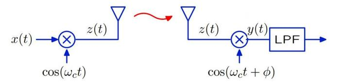
What happens if there is a phase shift  $\phi$  between the signal used to modulate and the one used to demodulate?
