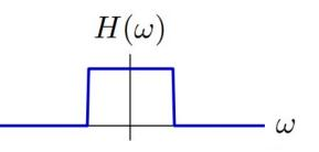
The **frequency response** is Fourier transform of **impulse response**!
