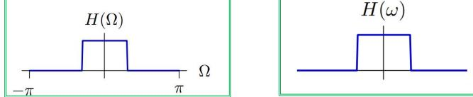
The **frequency response** is Fourier transform of **unit-sample/impulse response**!
