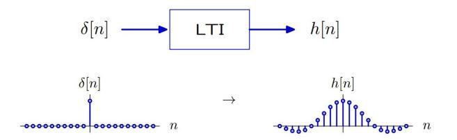
The unit-sample signal is the shortest possible non-trivial DT signal. It is the building block of any arbitrary DT signal x[n]:  $x[n] = \sum_{k=1}^{\infty} x[k] \delta[n-k]$
