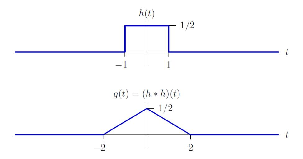
Convolution in time is equivalent to multiplication in frequency.
