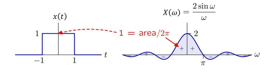
$$x(0) = \frac{1}{2\pi} \int_{-\infty}^{\infty} X(\omega) e^{j\omega 0} d\omega = \frac{1}{2\pi} \int_{-\infty}^{\infty} X(\omega) d\omega$$
