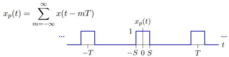
Since  $x_p(t)$  is periodic, it has a Fourier series (which depends on T) Find Fourier series coefficients  $X_p[k]$  and take the limit of  $X_p[k]$  as  $T \to \infty$ As  $T \to \infty$ ,  $x_p(t) \to x(t)$  and Fourier series will approach Fourier transform.
