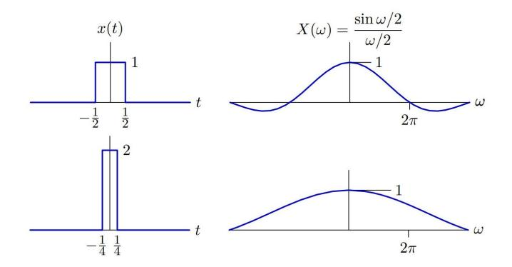
In the limit, the pulse has zero width but area 1! We represent this limit with the delta function:  $\delta(t)$ .
