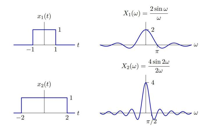
Stretching in time compresses in frequency.
