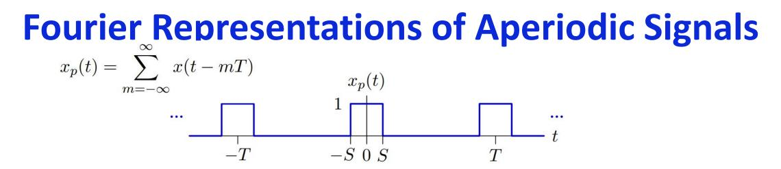
Calculate the Fourier series coefficients  $X_p[k]$ :
